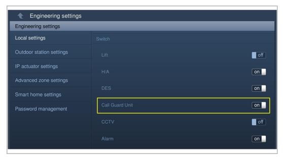
On the "Engineering settings", "Local settings" screen, the address of default guard unit must be set (the system default is 1).
